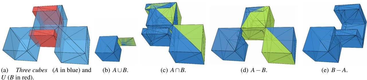
**Fig. 5** Boolean operations using *VTK* with *Three cubes* (model *A* in blue) and *U* (model *B* in red). For (b)-(e), blue is the outer facing and yellow-green is the inner facing.
