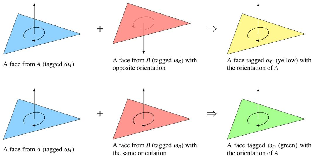
**Fig. 3** Applying tags  $\omega_C$  and  $\omega_D$  on duplicate faces. For duplicate faces, the face tagged  $\omega_B$  is removed and that tagged  $\omega_A$  changes to  $\omega_C$  or  $\omega_D$ .
