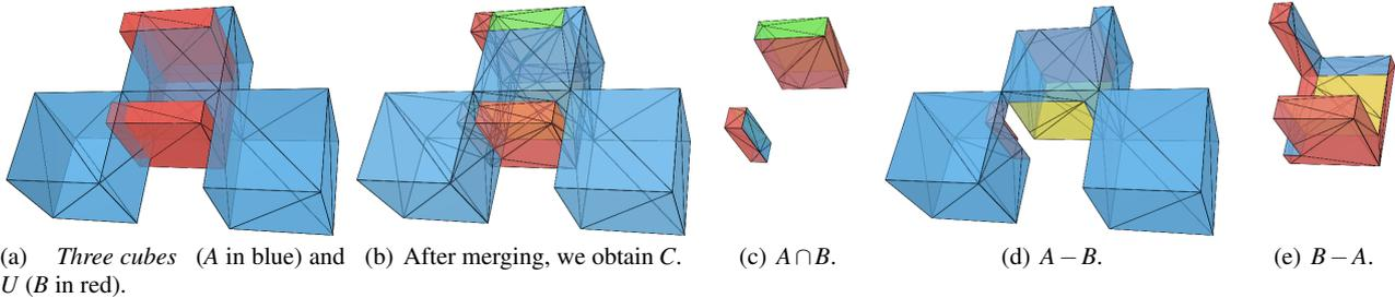
**Fig. 4** Boolean operations using *BORES* with *Three cubes* (model *A* in blue) and *U* (model *B* in red). Legend. clear blue: tag  $\omega_A$ , clear red: tag  $\omega_B$ , yellow: tag  $\omega_C$  and green: tag  $\omega_D$  (figure from [14]).
