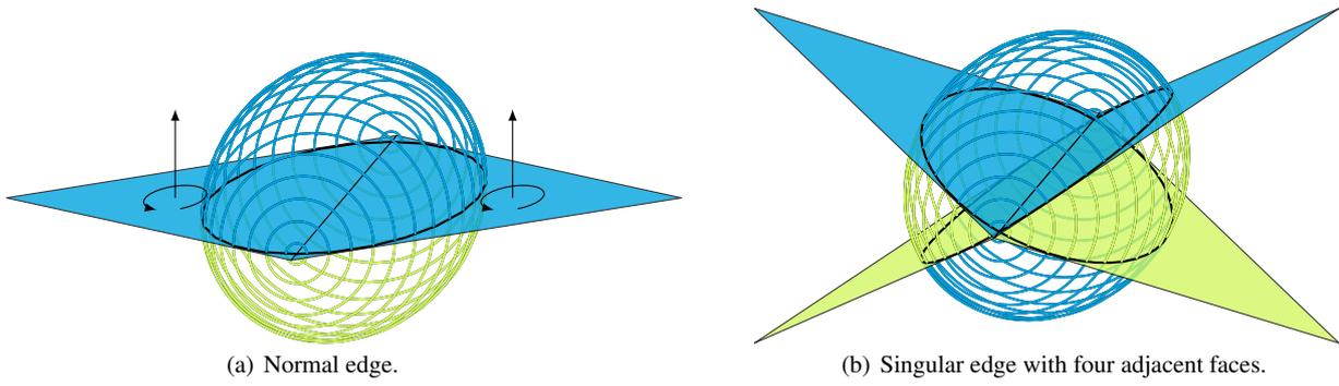
**Fig. 1** Examples of edges with consistent definition of the interior (green) / exterior (blue) (figure from [14]).
