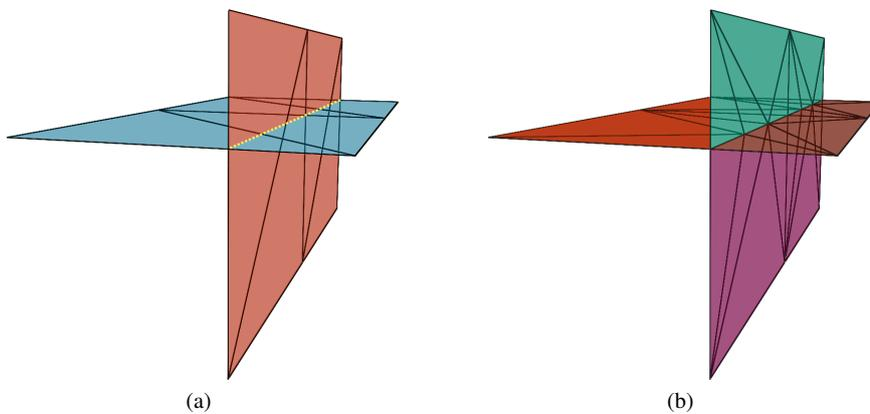
**Fig. 2** Simple example of intersection between two shells (figure from [14]). (a) Two shells (*A* in blue and *B* in red) are colliding. The yellow dotted line is the intersection line. (b) After computation and remeshing of intersections, we obtain *C*. *C* can be decomposed in patches rendered in different colours.
